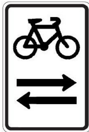
Example: Advanced Contra-flow cycle facility sign
